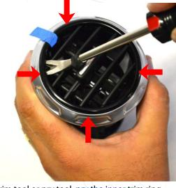
Using a trim tool or pry tool, pry the inner trim ring forward releasing the clips at the 4 locations shown.
