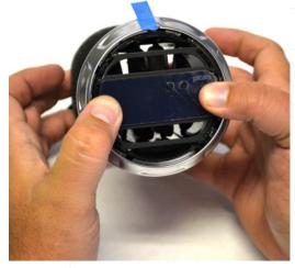
Line up the tabs of the metal display bracket to the vent slat positions. Center the gauge perfectly before applying pressure evenly to the sides of the gauge as shown.
