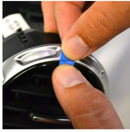
Rotate the ring of the gauge so that it is at the top and the vent is open. Mark the top of the OUTER and the INNER rings so that you can line them up again later.
