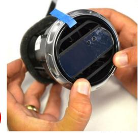
Apply pressure to the bottom clip locations as shown to seat the bottom clips. After the clips are seated you can remove any center markings you applied.
