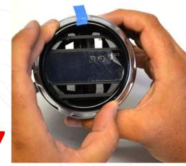
Line up the inner trim ring with the markings that we placed in step 1. Gently insert the ring with no force to get it lined up and seated but not yet clicked into place.
