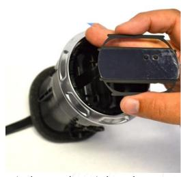
Feed the display cable connector and wire through the far left opening between the vertical vent slats. Feed the wire through and line up the gauge into the front of the vent. The top of the gauge has the logo and buttons, be sure the gauge is installed right side up.
