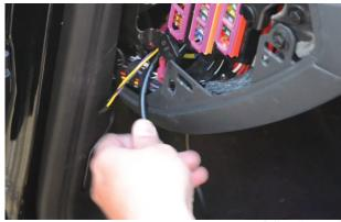
Tuck wires and control box into the dash. Secure them so that it does not fall out.
