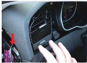
Insert the P3 VIDI pre-installed vent into the dash, running the wire out the side. If you did not order pre-installed, see vent install PDF file at p3cars.com/install
