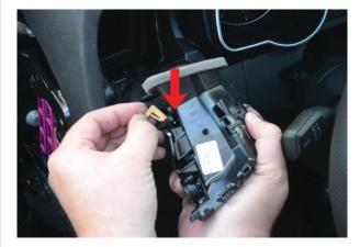
Carefully remove the vent and disconnect the small lighting connector
