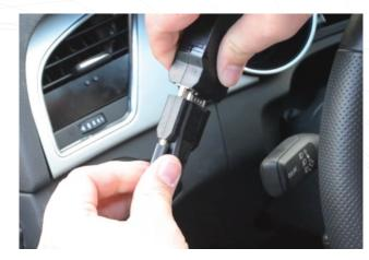
Connect the harness to the control box and tighten connectors.
