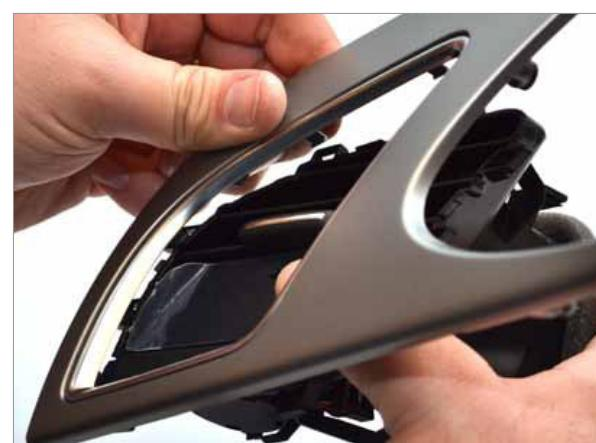
**9** Carefully re-attach the trim to the vent assembly. If you have trouble keeping the parts from falling out, you can use a temporary piece of tape across the right side to hold them in until the trim is in place.
