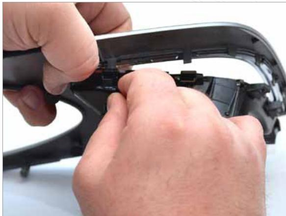
**1** Using a flat blade screwdriver, unclip the trim from the vent, be careful that the slats do not fall out.
