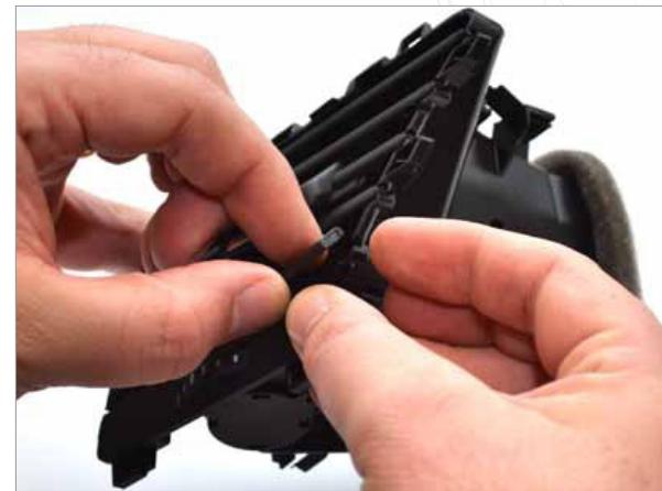
**4** Carefully remove ONLY the bottom slat starting on the side of the vent that is closest to the steering wheel.
