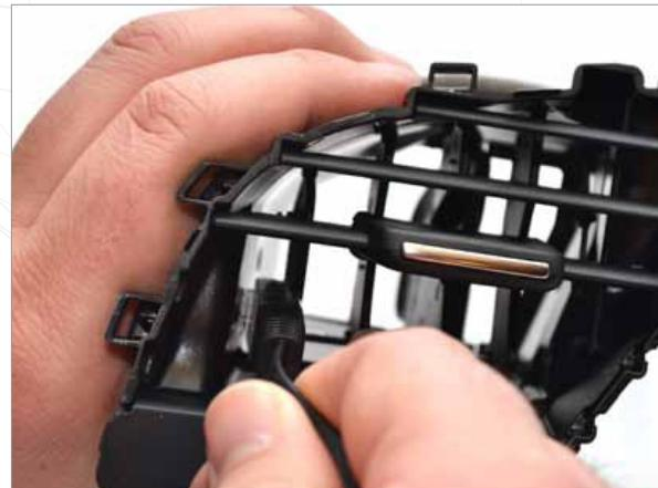
**7** Insert the wire in the vent by squeezing the connector through the left bottom corner as shown. Feed all the wire through.
