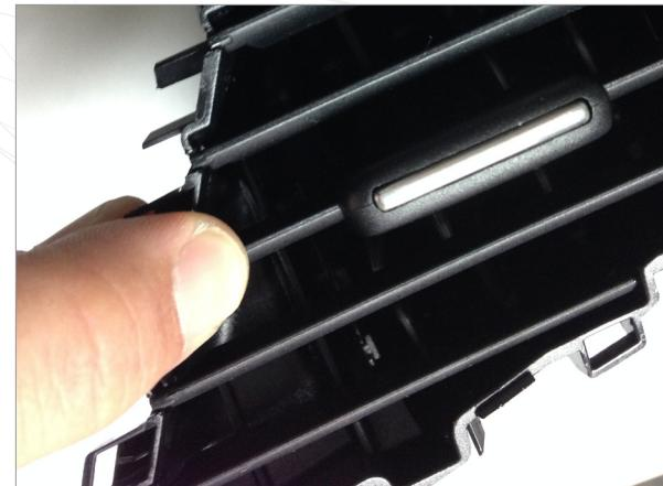
**2** Place index finger over the central control slat while removing lower slats. This will insure control and up slats remain in the vent and in union with one another.
