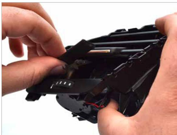
**5** Now remove the second from bottom slat, this slat will have a small metal controller bar behind it that will need to unhook from the slat above it as it comes out. Once again, take care that the other slats do not come out.
