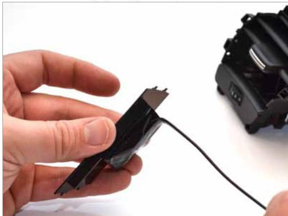
**6** Prepare the display unit, make sure the wire comes off the back at a 90 degree angle.
