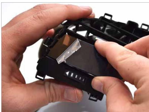
**8** Peel the protective covering off both sides of the glass face so the tabs are not covered. Insert the tabs on the glass into the holes on the vent as shown here starting with the far side. The gauge should rest inside the slots where the vent slates were before. If the gauge will not sit flush, check that the wire is positioned properly.
