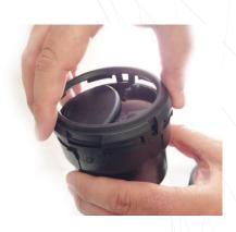
Feed the VIDI display cable through one of the outer holes on the vent tube rear.
