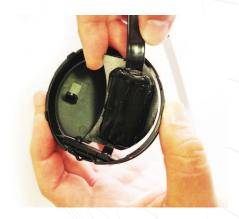
Insert the VIDI Display into the carraige. The 2 small tabs fit into the HOLES where the old double flap vent peice was retained. Once again, sqeeze the vent ring on the top and bottom to flex it and allow easy insertion.
