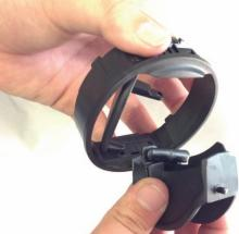
Remove the connecting arm from the top flap, and remove the bottom double flap to create room for the gauge. You can squeeze the top and bottom of the circle to flex it open and easily remove the vent flaps.
