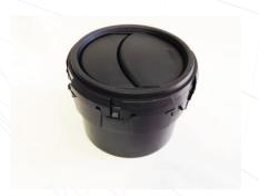
Remove the largest outer trim ring by releasing the clips on the sides of the vent.
