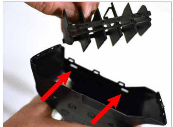
**4b** Also unclip the inner vent slats from the tube. You can flex the vent vertically and release them.
