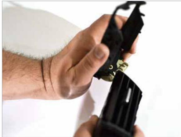
**3** Pull down and forward until the bottom clips release and the entire front cover of the vent will come off.
