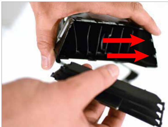
**4a** Unclip and remove the vent slats from the vent.
