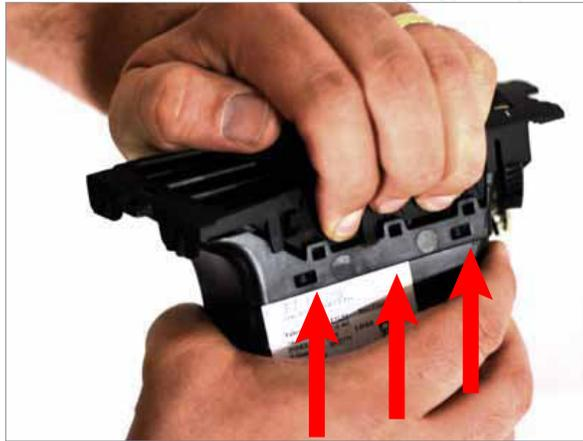
**1** Unclip the 3 top clips of the vent as shown. You can simply put pressure between the clips and pull forward.
