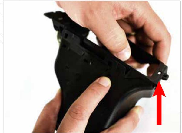
**2** Unclip the front clip on the right side of the vent and flex the front of the vent forward.
