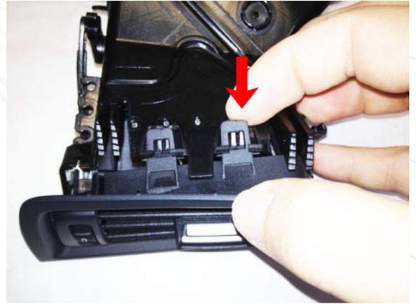
**2** Push forward as you release the clips to slide the catch over the retainer
