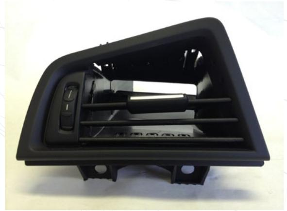
**7** Fully re-unite the vent front with the rear hosing and make sure the remaining bottom 3 slats are installed correctly and move up and down as intended.
