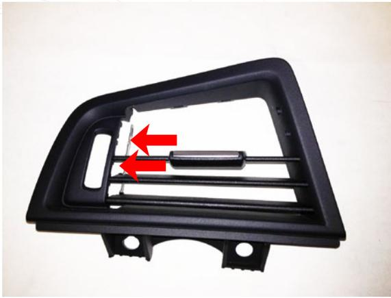
**6** On the vent face, carefully remove the top two slats, taking care to leave the remaining 3 slats in their proper position and still connected with the vertical metal positioner.
