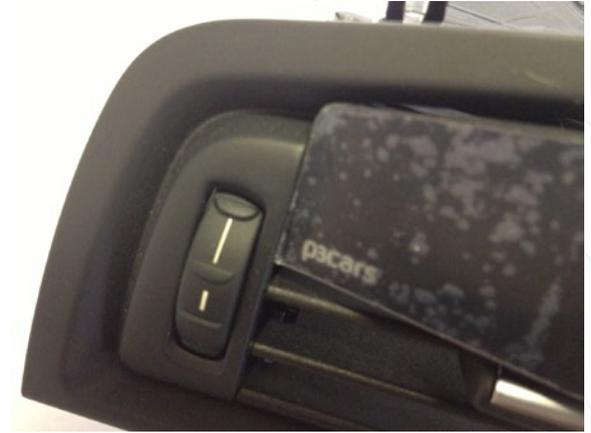
**9** Insert the side of the display shown here into the un-occupied vent slat holes from the vent slats we removed.
