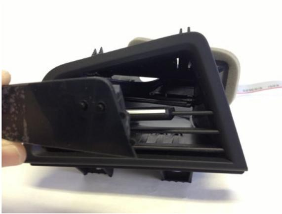
**8** Feed the cable from the p3 VIDi display unit through the top rear of the vent.
