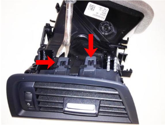
**1** Release the clips on the top of the vent with your finger or a trim pry tool.
