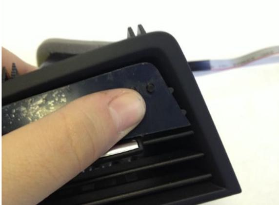
**10** Apply pressure to the other side of the VIDi display unit to complete the installation. Pressing the display in and towards the driver side will make it pop in easily.
