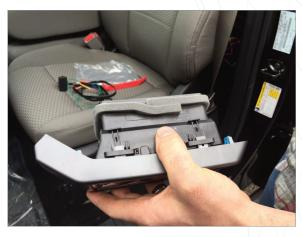
Next remove vent facia trim by releasing the clips on the side of the vent housing.
