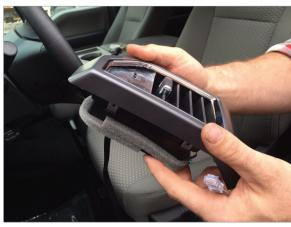
Place your vehicles trim on the vent with the P3 Cars VIDI or P3 Boost Gauge installed.
