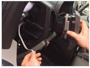
Feed display cable through the dash vent opening and down the side dash area.
