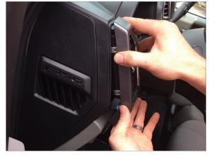
Remove vent housing by pulling straight out with a slight upward motion.
