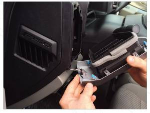
Disconnect the connector at the bottom of the vent housing.
