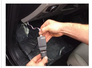
Connect display cable to control box.
