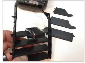
Remove the top 3 horizontal slats from the vent slat assembly.
