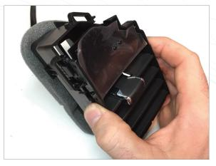
With the horizontal slider all the way to the left and vertical slats all the way open, reinstall the slat assembly with display. (Feed display wire through the slot cut in step 5)
