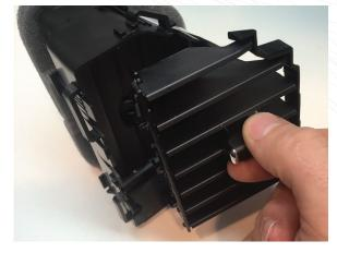
Remove horizontal slat assembly from the vent housing.
