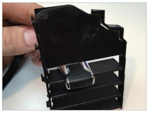
Insert display into the vent slat assembly.
