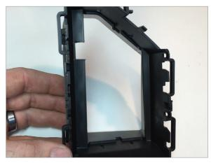
Measure down 1" from the top of the vent housing and cut a 7/16" slot as shown in picture.
