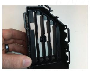
Reinstall vertical slat assembly into vent housing.
