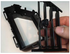
Remove the vertical slat assembly from the vent housing.
