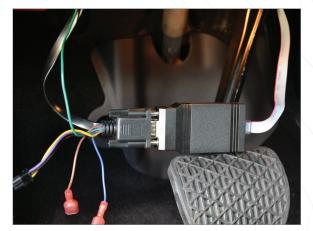
Route both the OBD2 cable and the display cable to the back of the lower dash trim just above the brake pedal and to the right of the hood release. Connect both cables to control box. (Be sure not to allow cables to interfere any moving parts such as the brake/gas pedals and steering column)
