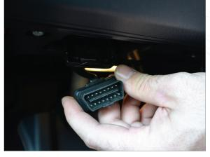
Drop OBD2 connector down just behind OBD2 port to the right of the hood release. Firmly connect OBD2 connector to the OBD2 port.
