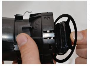
Taking note of where the top of the housing is, ("Top" is molded into the housing) install the display in the housing so that it will be level when installed in vehicle.
