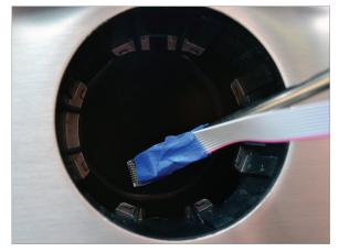
Using a long screwdriver or coat hanger, feed the display cable throught the gap toward the gas pedal.
