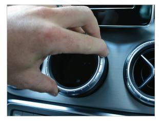
While gently pulling the end of the display cable to take out slack, install the housing back into the trim.
