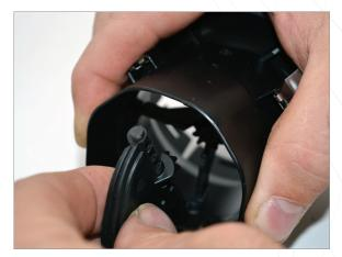
Squeeze the housing to elongate and remove the flaps.
