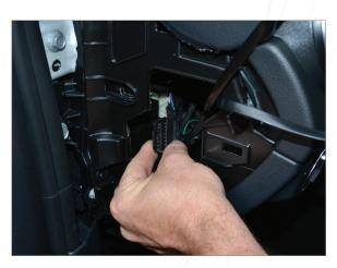
Feed the OBD2 end of the OBD2 harness back down through the dash toward the brake pedal.
