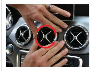
Rotate trim ring counter-clockwise and remove.
