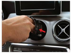
With a firm pull, remove the housing from the dash trim.
