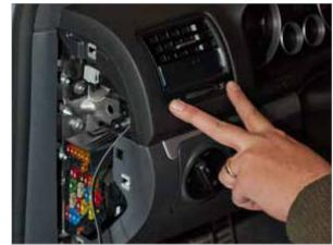
Push on the bottom corners of the vent to firmly secure into place.
