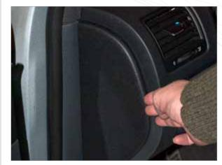
Open the driver's side door and remove the cover to the fuse box.
