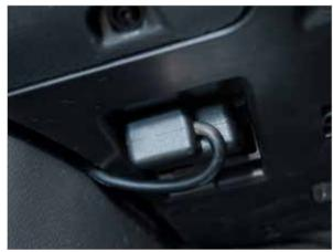
Plug the connector firmly into your cars diagnostic port. Tuck any visible cord into the creases.
