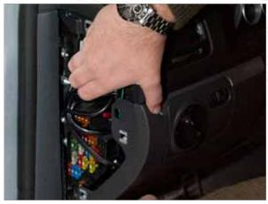
Tuck the control unit and the remaining cable into the fuse box. Make sure the cable that will be plugged in into the diagnostic port is tucked into the crease at the bottom of the fuse box.
