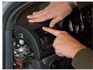
Pull the entire cable through the fuse box and snap the new vent into place starting at the top.
