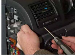
Use your fingers to push out the lower left corner of the vent and insert a screw driver to pop out from the bottom up.
