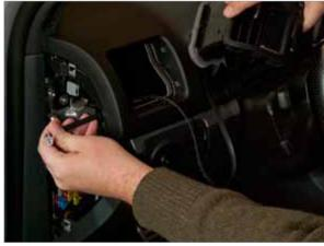
Thread gauge connection cable through the vent opening and out the fuse box.
