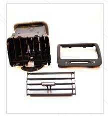
Prepare the vent. Using a flathead screwdriver, unclip the vent face starting with the bottom clips. You may need to rotate the open/close dial to gain access to the lower clips. Press down and forward to slide the bottom clips out.
