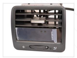
Insert the slats assembly into the vent, lining up the tabs and slat controller, it will fit snugly. Feed the wire through as shown, you may need to kink the wire at a 90 degree angle to keep the wire in place. Line up the glass onto the vent, press to adhere it to the front of the vent frame as shown. After you verify the gauge is fitted as shown, slide on the front of the vent until all 4 clips click into place.
