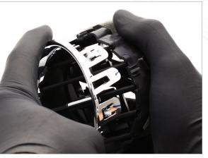
Release tabs on trim ring to remove it from vent housing.
