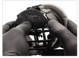
Install display into vent housing.
