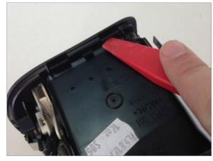
On bottom of the vent housing release the right most clip.
