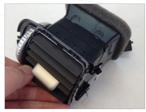
You will now be removing the bottom 3 horizontal vent slats. Unclip the slat under the left right control starting at the left most part of the vent housing.
