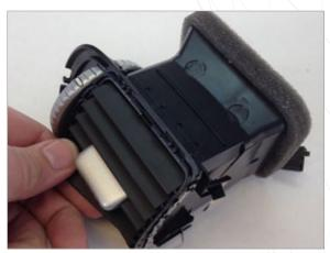
Remove the bottom horizontal vent slat.
