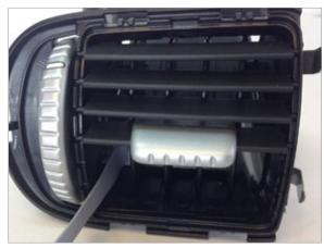
Feed in the display cable between the left most wall of the vent housing and the left most vertical vent slat as shown.
