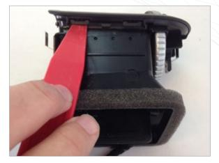
Starting on top of the vent release the left most tab connecting the Facia trim to the vent housing.
