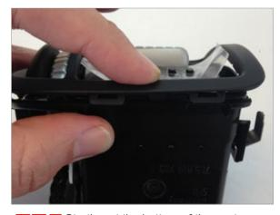
Starting at the bottom of the vent reattach the Facia trip. Ensure the VIDI's protective covering does not get pinched. This will prevent you from being able to cleanly remove the protective covering.
