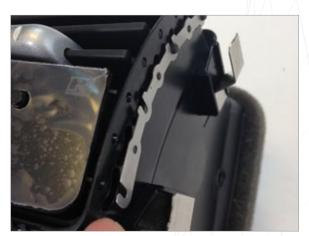
Insert the P3 Cars VIDI right side first. Ensure that the aluminum bracket tabs are in the top and bottom empty vent slat holes as shown.
