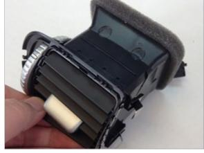
Remove the next to last horizontal vent slat.
