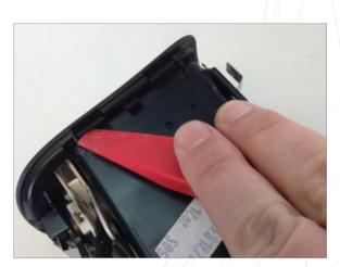
Release the final clip connecting the Facia trim to the vent housing.
