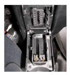
Feed display cable on your VIDI into the vent cavity and to the left.
