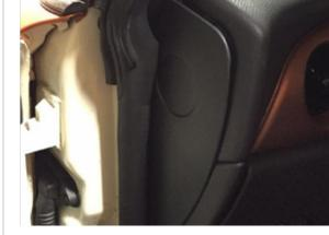
Using your finger or a soft trim pry tool open the side dash cover panel.
