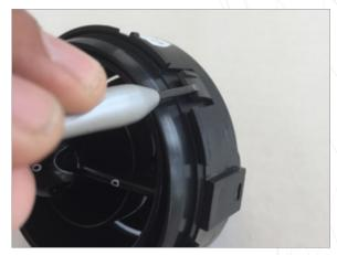
Slide a very small flat head screw driver in the middle of each tab where it is open and between the two grab clips that are on each tab as shown.
