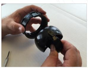
Removed the inner vent housing from the outer vent housing.
