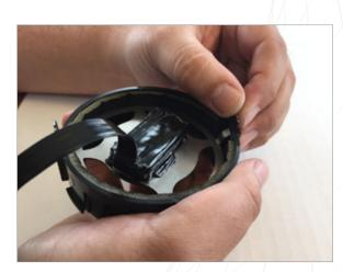
Once past the foam insert the side clip into the retainer clip in the side of the vent housing wall.
