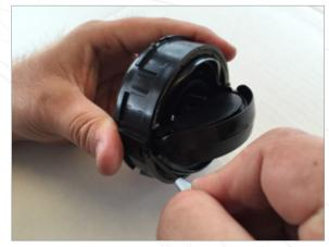
Release the clip on the right side of the vent housing.
