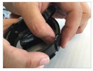
Insert the other side clip into the retainer clip in the side of the vent housing wall.
