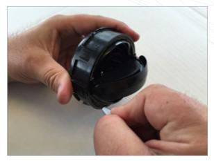
With a micro size flat head screw driver release the clip on the left side of the vent housing. It will slide out of it's housing slightly.
