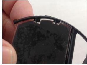
Insert the VIDI display into the retainer clip on the left.
