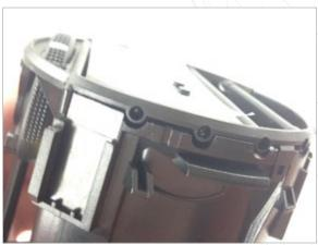
Reinstall the horizontal slat retainer assembly with the VIDI now installed.
