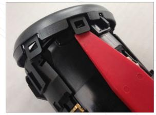
Release the final clip connecting vent facia to the vent housing.
