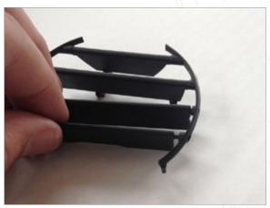
Release the clip holding the horizontal vent slats.
