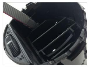
Feed display cable in on far left side of vent between the vent wall and the last vertical slat.
