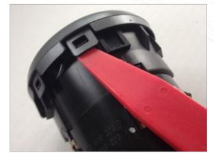
Release the clips on connecting the vent facia to the vent housing.
