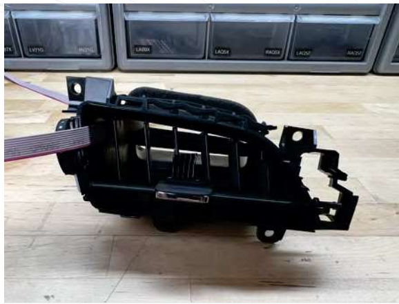
6a Feed ribbon cable through left side of vent with pink side on bottom
