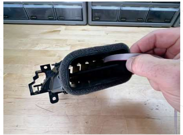
6b Make sure cable is flat against vent housing
