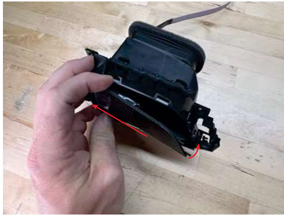
7 Install display by aligning left pegs with holes in vent then rotating right side of display into place
