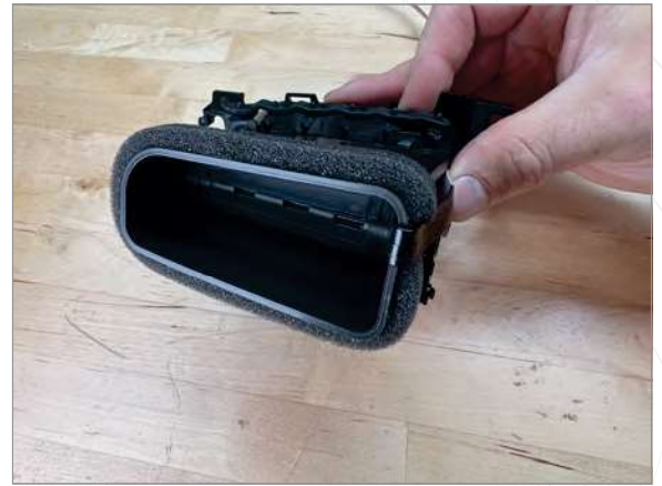
8 Close vent flap to hold cable in place. Pinch cable around back of vent as shown
