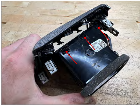
1a Remove trim from vent housing by releasing 3 clips on the top of the vent
