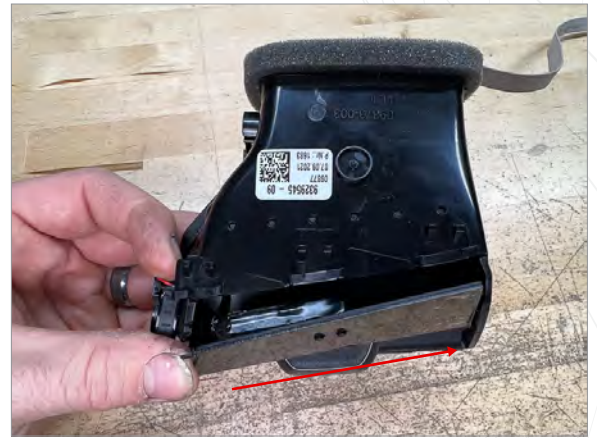
7a Install display by sliding right alignment pegs into corresponding holes in vent housing
