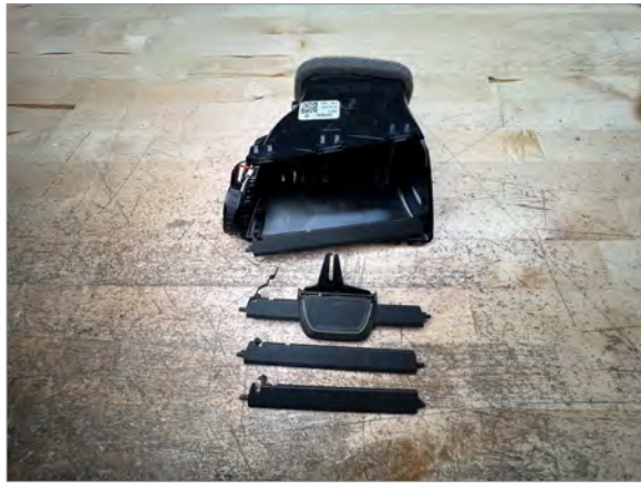
2 Remove the slats from the vent housing by pulling out on the left side of each slat
