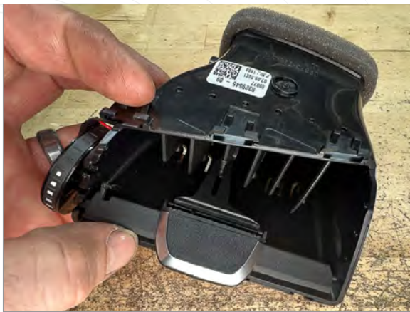
5 Reinstall bottom slat, making sure to line up vertical slat control fork as shown
