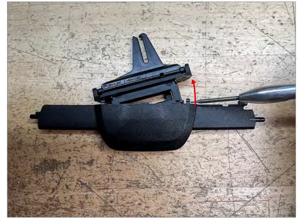
3a Remove the slider from the third slat by prying on side clips as shown
