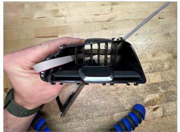
6a Route the ribbon cable between the leftmost vertical slat and the vent housing feeding it below the airflow control flap
