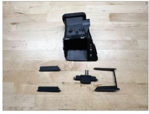
Remove 3 center slats from slat assembly and keep in order as shown. Upper removed center slat will not be reused. Middle slat will be used in step
