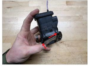
Insert right side of display into slat holes, then rotate display into place.
