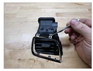
Using a small screwdriver, release the 9 clips around the trim to remove it.
