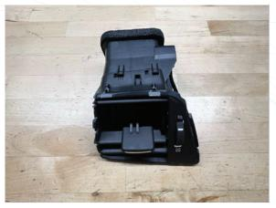
Reinstall slat assembly making sure slider fork properly engages with vertical slats for left/right movement.
