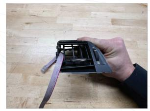
Feed display cable through vent as shown. (pink side down, cable flat against housing)
