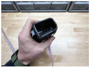
Fold display cable around back of vent as shown and close flap to hold in place.
