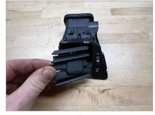
Remove slat assembly as shown.
