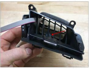
When installing vent slat be sure to line up control fork with vertical slat pin. Feed the ribbon cable through the vent as shown.
