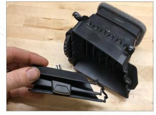
Use a small screwdriver or pry tool to remove vent slat assembly from vent housing.
