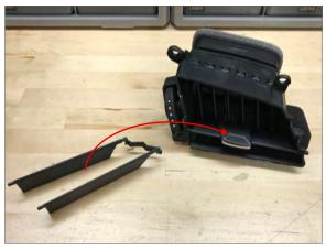
Remove center vent slat and reinstall it into bottom vent slat position.
