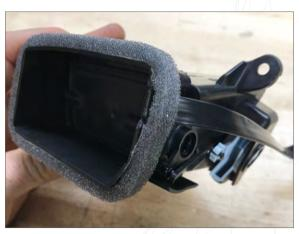
Cut foam away from vent housing and feed cable through as shown.
