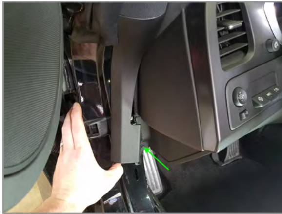
9 Remove screw behind trim panel next to door
