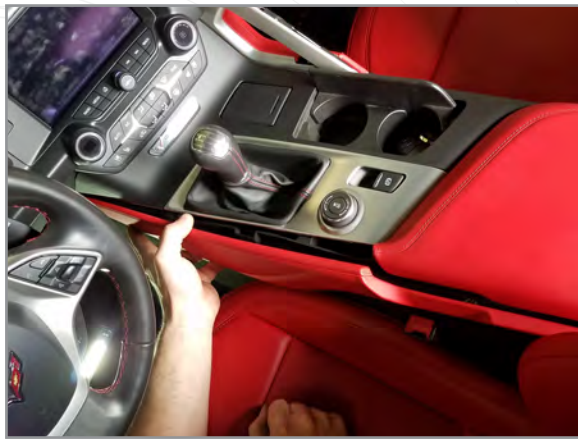
7 Remove console trim and set aside
