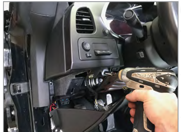
12 Remove dash trim screw as shown
