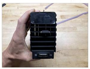
Reinstall slat assembly into housing
