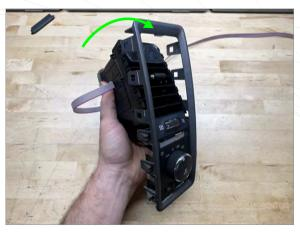
Roll vent back into trim and make sure all clips are secure (Bottom of vent overlaps trim)
