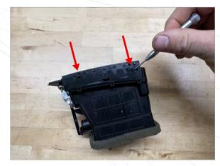
Release 2 clips and remove slat assembly from housing.
