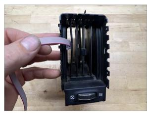
Feed display cable through left side of vent (May need to bow slat)
