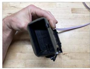
Close air flap, then fold display cable around back of vent housing as shown
