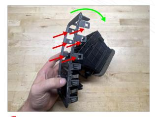
Release 6 clips and rotate vent out of trim as shown
