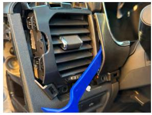
Use a pry tool to move cluster bezel out of the way, then slide the vent out
