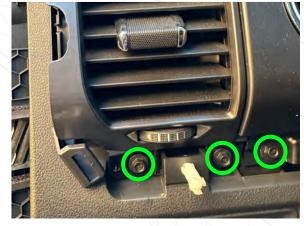
Remove 3 7mm fasteners
