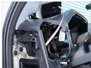
Feed display cable through dash and to plug into control box. Plug control box into OBD2 connector and tuck in lower dash.
