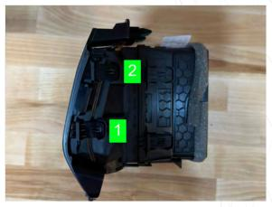
Remove the faceplate from the vent by releasing the 7 tabs that secure it to the vent with a flat pry tool
