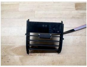
Install display into horizontal slat assembly
