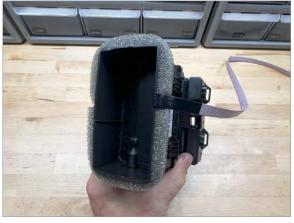
Fold display cable around back of vent and close air flap to hold it in place
