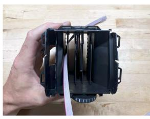
Feed the display cable through the vent housing as shown (Be sure to keep cable flat on left side of vent housing)
