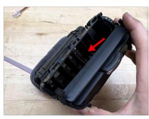
Install slat assembly back into vent housing (Make sure handle fork engages correct vertical slat)
