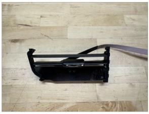
Install display into slat assembly
