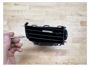
Use small flathead screwdriver to remove slat assembly from vent housing
