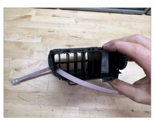
Feed ribbon cable through bottom left of vent housing (keep cable flat and ensure pink side faces down)
