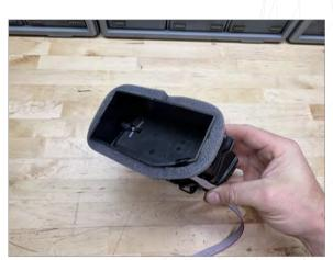
Fold ribbon cable around back side of vent as shown (optional: can be tucked under foam)
