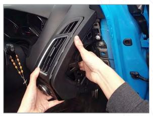
Partially disengage vent assembly from dash trim by sliding towards driver seat.
