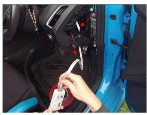
Remove the storage compartment and route the display cable as shown by the red arrows. Connect display cable to control box.
