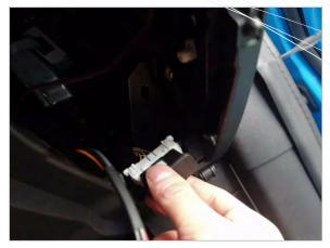
Plug the gauge into the vehicle's OBD2 port and start engine to test functionality BEFORE installation
