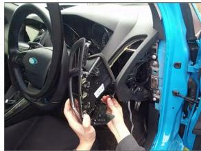
Position the air vent in preparation to reinstall it back into the dash trim. Plug connector from dash trim back into head lamp control panel.
