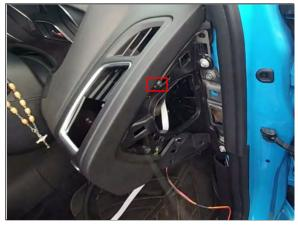
Replace the T20 Torx screw to secure the vent to the dash trim.
