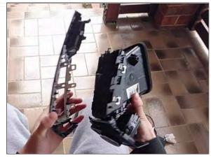
After all clips are released, separate the facia from the vent.
