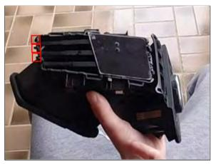
Insert the display tabs into the existing vent groves.
