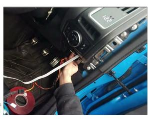
Plug in the OBDII cable from the P3
