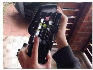
With a flat-edged trim tool, push the vertical vent slats from behind the slats outwards, being careful only to exert enough force to "pop" them out.
