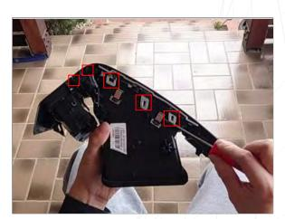
Release clips to remove vent facia from vent. There are 5 on each side.
