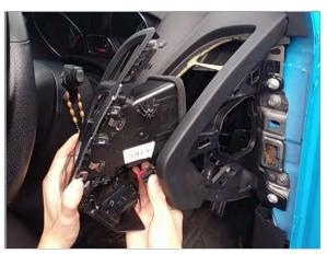
Unplug connector from headlamp control panel underneath the air vent. Then fully remove the air vent from dash trim.
