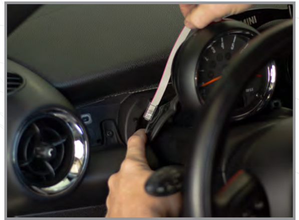
6b Feed the display cable through the hole and out the side of the dash
