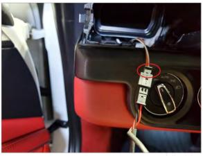
Unclip the connector for the lighted vent wheel.
