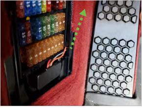
Feed OBD2 harness through opening in fuse box and out from behind carpet (OBD2 Harness can be seen in step 6.) Connect to main harness and control box. Then plug OBD2 connector into port.
