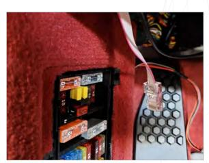
Feed the display cable down to the fuse panel in the driver's footwell and connect to the control box
