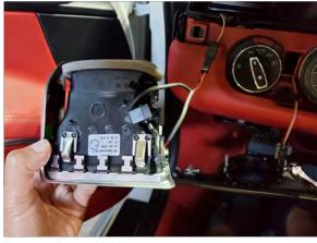
Pull the vent straight back towards the driver to remove it from the dash
