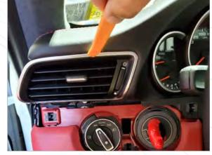
Use a trim tool to loosen the vent from its place in the dash
