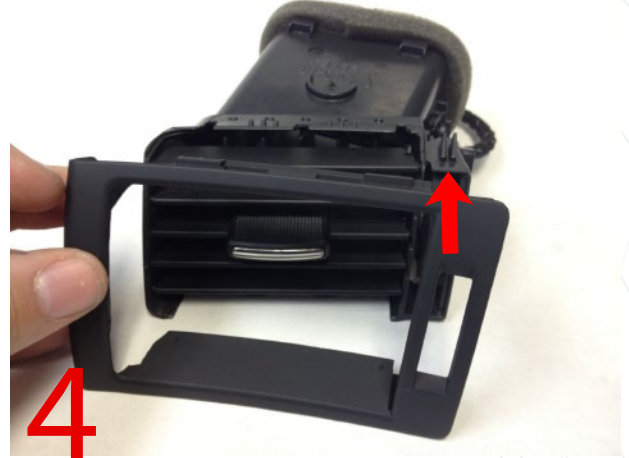
4 After all clips are free the face will come off.
