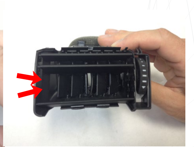
5 Remove the center slat with the controller, along with the slat directly below it so that your vent looks like the one shown on the right with 2 missing slats.
