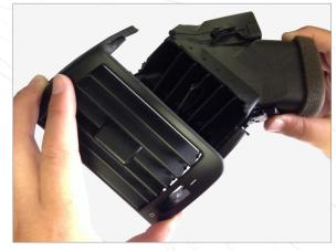
Bend down and forward to break lower bonds and unclip clips.
