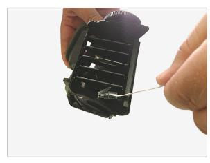
Feed cable in left most side of vent against vent housing wall.
