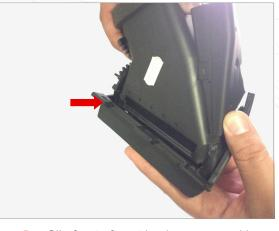
Clip front of vent back on rear making sure all seams line up and that lower outer clip is not tucked inside rear of vent housing.
