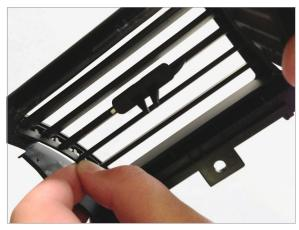
Remove bottom two vent slats from the vent slat keeper.
