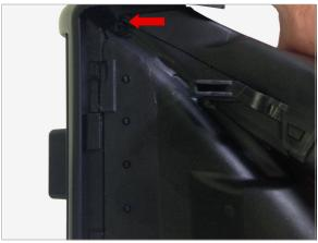
With an hi temp epoxy re bind the front and rear of vent housing at union joint.
