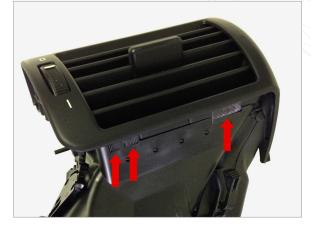
Use an exacto knife cut a line thru the three seam welded regions on the top of the vent.
