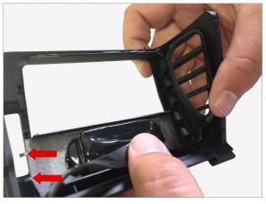
Install P3Cars gauge into the bottom vent clips left side first and then right side. Make sure clips are seated in these notches.
