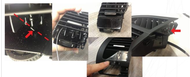
Trim the small tab that protrudes into the area where the VIDI display will sit. Feed the display cable through the far side of the vent and out the back. Place the display in the place of the 2 lower slats. Replace the vent facia and secure the rear plastic tab with a hot iron or glue.
