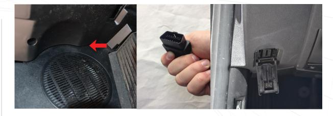
Route the HD15 side of the harness connector through the slot show in RED and out the vent opening. Plug the dianostics connector into the OBD2 Port.
