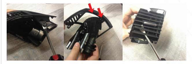
Pop the plastic tab on the back of the vent, and release the 2 clips on the left side of the vent. Remove the entire vent facia, and then pop out the BOTTOM TWO vent slats ONLY.
