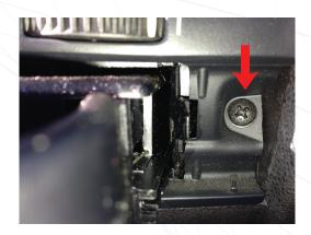
Remove the retainer screws holding in the vent and remove the vent from the vehicle. You will need to unscrew the 2 screws shown, remove the vent and cupholder assembly, and then remove the cupholder by unscrewing the TORX screw on the rear of the vent
