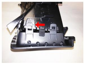
Repeat the clip releasing procedure on the sides and bottom of the vent.
