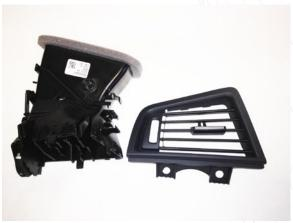
Work your way around the vent releasing all clips until the front face of the vent is free.
