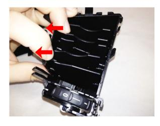
Using your fingers flex the top of the vent upwards to release all of the inner vertical slats of the vent. After all inner slats are removed set them aside in a safe place in case you wish to return your vent to stock.
