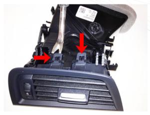
Release the clips on the top of the vent with your finger or a trim pry tool.
