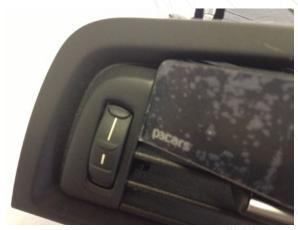
Insert the side of the display shown here into the un-occupied vent slat holes from the vent slats we removed.
