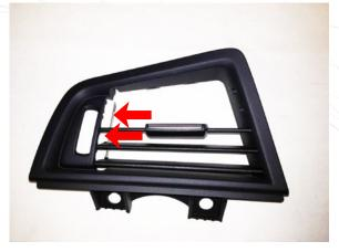
On the vent face, carefully remove the top two slats, taking care to leave the remaining 3 slats in there proper position and still connected with the vertical metal positioner.
