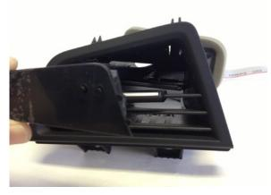
Feed the the cable from the p3 VIDI display unit through the top rear of the vent.
