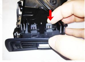
Push forward as you release the clips to slide the catch over the retainer
