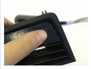
Apply pressure to the other side of the VIDI display unit to complete the installation. Pressing the display in and towards the driver side will make it pop in easily.
