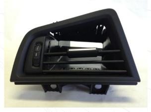
Fully re-unite the vent front with the rear hosing and make sure the remaining bottom 3 slats are installed correctly and move up and down as intented.
