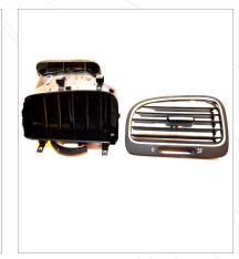
Prepare the vent. Using a flat head screwdriver, unclip the vent face starting with the bottom clips. You may need to rotate the open/close dial to gain access to the lower clips. Wedge the screwdriver behind the vent front at the tab and force it over the tab.
