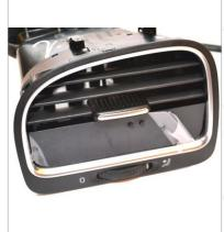
Feed the gauge wire through the far left slat, and line up the slat controller onto the inner slat bar before clipping the vent back together. You may need to clip the left side of the vent last to get all the clips to fasten.
