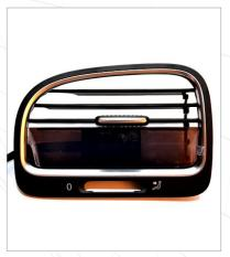
Insert the glass into the vent face from behind, make sure the bottom lip of the glass is OVER the bottom ridge of the vent face as shown in the photos below. Clip the slat assembly back into the vent face from behind, pinching the gauge glass in place.
