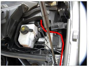
**15** From inside the car, feed 8-12 inches of nylon tubing and coat hanger from step 13 through the conduit hole. Then you will be able to see it pop out under the cover you removed in the engine bay, next to the wire harness, route it as shown. Disconnect the coat hanger, and get some slack.
