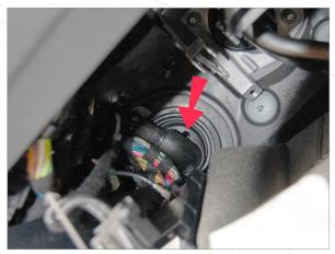
**13** Take the thin nylon boost tubing out of its package, and disconnect it from other hoses. Take a section of a coat hanger, or wire fish tool, and tape the tube to it. Poke a hole through the conduit shown at the extra tiny "tunnel" which is above the clutch pedal. Use a tiny screwdriver.
