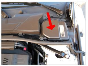
Pop the hood, and remove the driver side cover which hides the brake fluid reseviour. This cover just has clips on either side, and a rubber tab that hold it in place. After removing this cover, set it aside, this is all you need to remove in the engine bay area.
