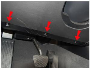
12 Go back out to the car, and remove the lower dash cover below the steering wheel by removing the three #20 torx screws shown above. Then lay this cover into the footwell.
